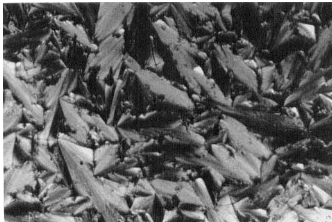
Figure 2. Optical texture of smectic A phase observed with a polarizing microscope ( \times 140 ) at 171^\circ\text{C} for 7-(4'- n -tetradecyloxybenzoyloxy) isoflavone.
